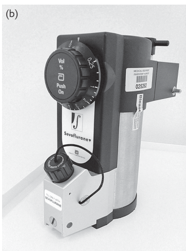
Fig 1.4b Yellow-coded vaporizers contain sevoflurane. The contents gauge is just out of sight on the left underneath the filling cap.
