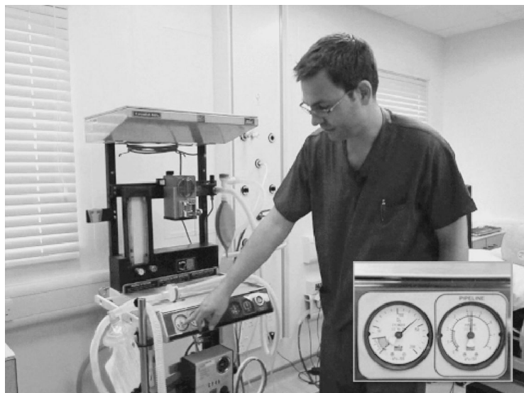
Fig 1.15 This demonstrates how to check an anaesthetic machine using the sequence taken from the Association of Anaesthetists of Great Britain and Ireland Machine Checks guidance document. There are several major steps, including power supply (00.11), gas supplies and suction (00.31), breathing system (02.39), ventilator (05.50), scavenging, monitors, and airway equipment (all at 06.44). A video of this is available in the video appendix.
